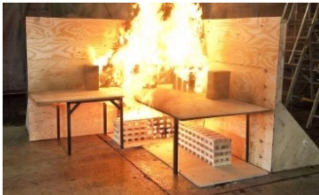
Tests simulated a typical office fire load
