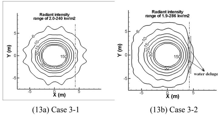
Fig. 13. Comparison of radiation heat flux distribution at  $Z=4.0\text{m}$  (Scenario 3).
