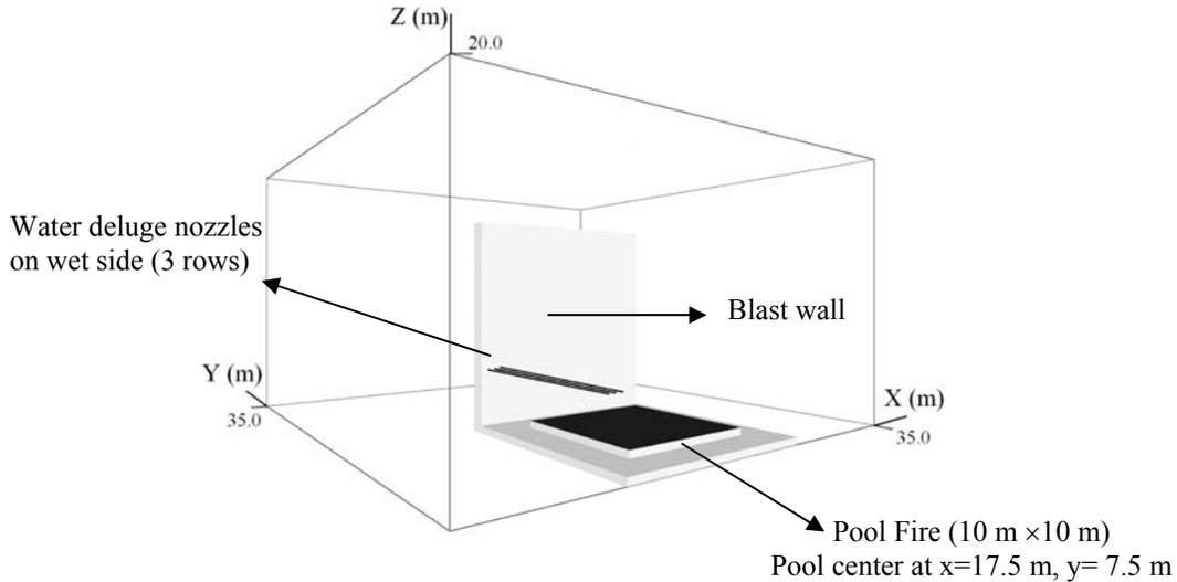
Fig. 2. Schematic diagram of Scenario 2.
