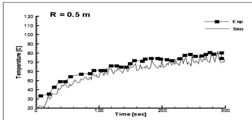
Fig. 4. Experimental and predicted temperature along the ceiling at  $R=0.5$  m (Scenario 1, no water deluge).
