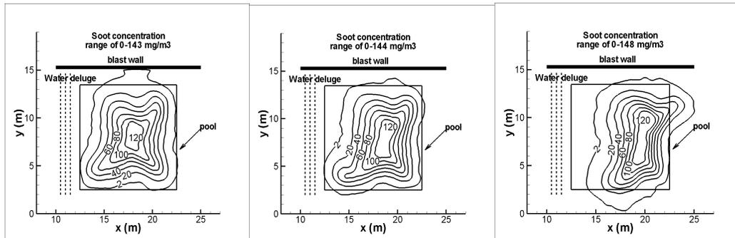
(8a) Case 2-1-2 (10 l/min/nozzle) (8b) Case 2-1-3 (20 l/min/nozzle) (8c) Case 2-1-4 (40 l/min/nozzle)
