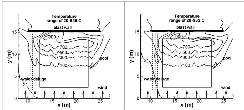
(12a) Case 2-4-3 (1800  $\mu\text{m}$ ) (12b) Case 2-4-4 (1000  $\mu\text{m}$ ), 16 m/s
