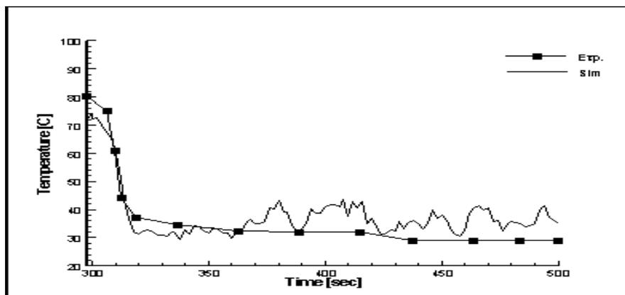
Fig. 5. Variation of mean ceiling temperature after water deluge activation (Scenario 1).
