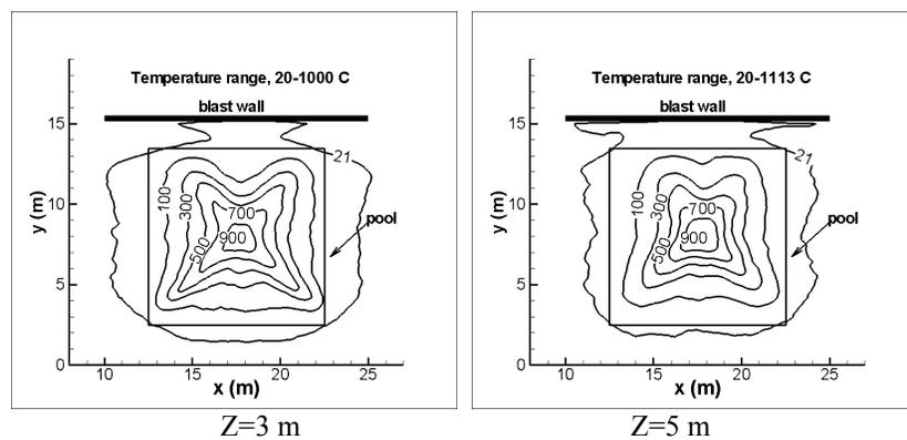
Fig. 6. Time-average temperature distributions at  $Z=3$  m and  $Z=5$  m above pool surface (Scenario 2, case 2-1-1, no deluge).
