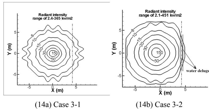
Fig. 14. Comparison of radiation heat flux distribution at  $Z=8\text{ m}$  (Scenario 3).
